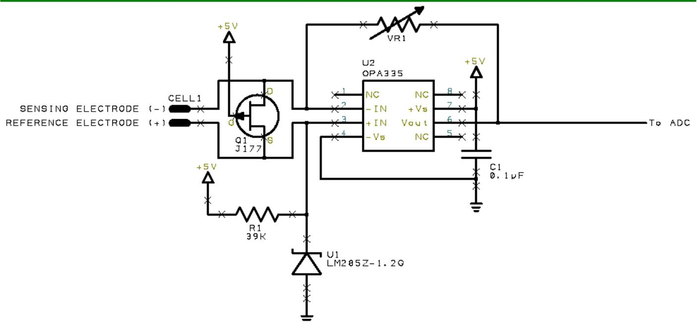
The reference circuit above is available pre-built from Dart Sensors for development purposes. It incorporates a JFET to short the sensor, preventing offsets from building up when not in use. It also generates a virtual ground, a requirement when operating in single-supply environments.
