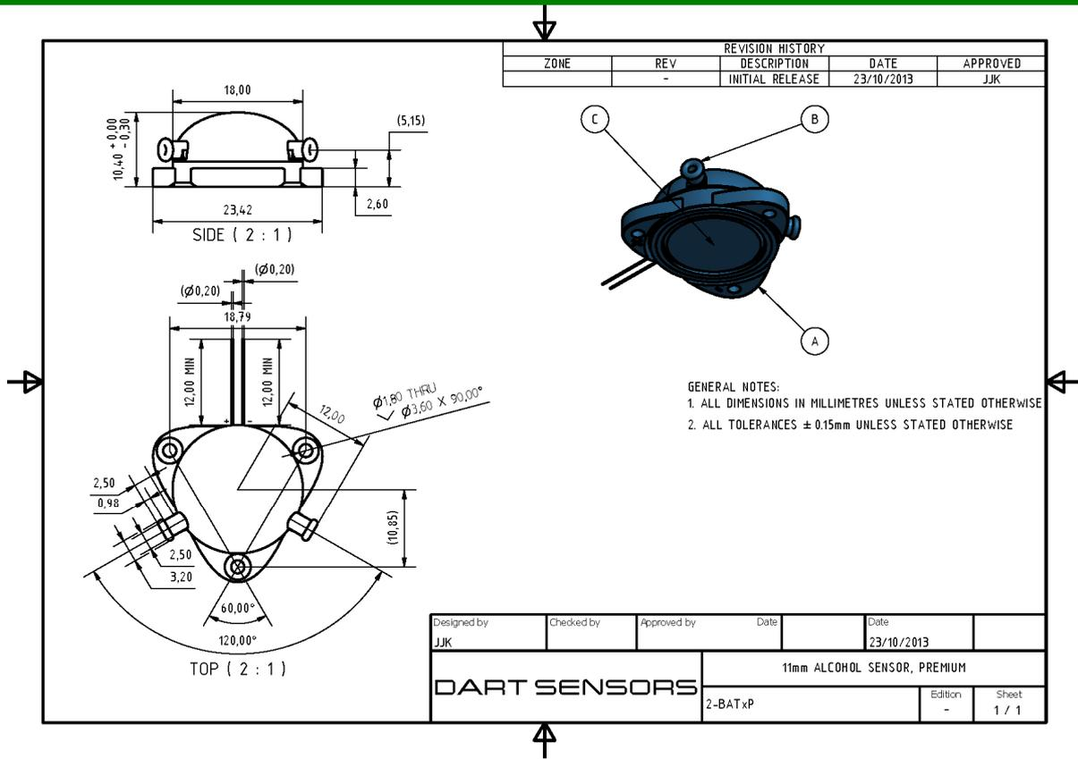
2-BATxE (economy sensors) are externally identical to 2-BATxP except connector wires are 0.15mm diameter.
